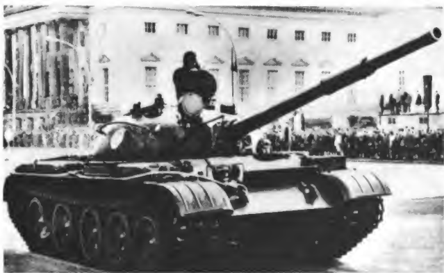
Figure 6-15. T-62 medium tank. The T-62, with a 115-mm smoothbore gun, is replacing the older T-54/55 as the Soviet main battle tank. It can be easily recognized by its five evenly-spaced roadwheels and the bulging fume extractor near the middle of the gun barrel.
